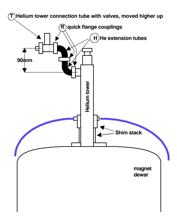
Lifting up the helium tower connection tubes.
