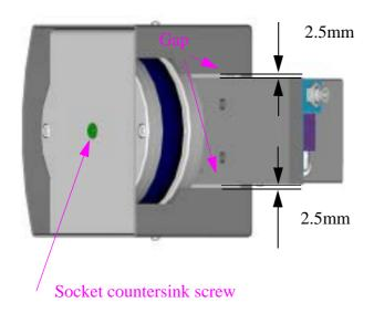
Before you unscrew the covers you have to check the correct position of the rubber bumper. To do this you have to turn it upside down and check the distance (gap) between the cover and the fixture part to the magnet stand. The gap to the cover should be equal (approx. 2.5mm) on both sides. You can adjust the position using the countersink screw.
