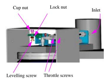
Switch the gas supply on and adjust the pressure reducing valve to approx. 5 bar. The gas supply must always be 0.5 -1 bar higher than the regulated gas behind the pressure reducer valve.
