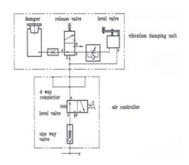
The accompanying diagram shows the pneumatic control box (air controller) and the pneumatic bumpers (vibration damping unit).
