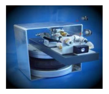
The throttle-valves are preset, opened by 1.5 turns. Do not alter this setting!
