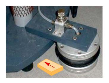
Only pneumatic vibration damping systems with a seperate pressure regulator valve can be upgraded to the newest self-leveling system (see photograph).
