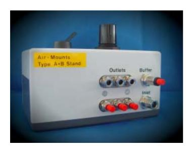
The pneumatic control box has one gas supply inlet and a total of 6 outlets for the pneumatic bumpers.
