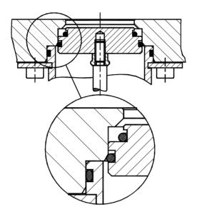
sealing plug inserted completly
