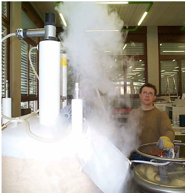
Figure 2.3. Provide Adequate Ventilation During Refilling
