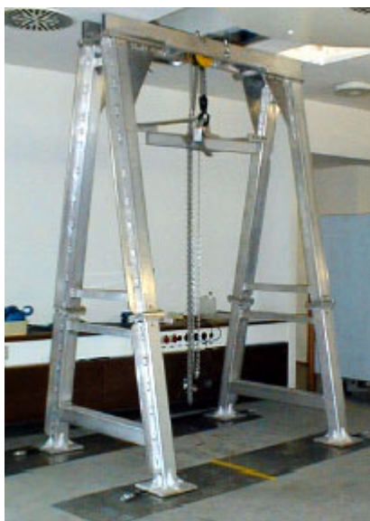
Figure 14.2. Bruker BioSpin - Special Rigging Equipment - The A-Frame
