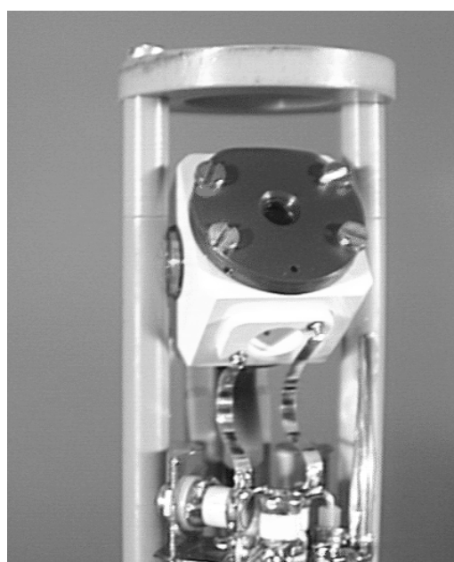
Figure 2.1. Upper probe chamber with MAS stator in magic angle position.
