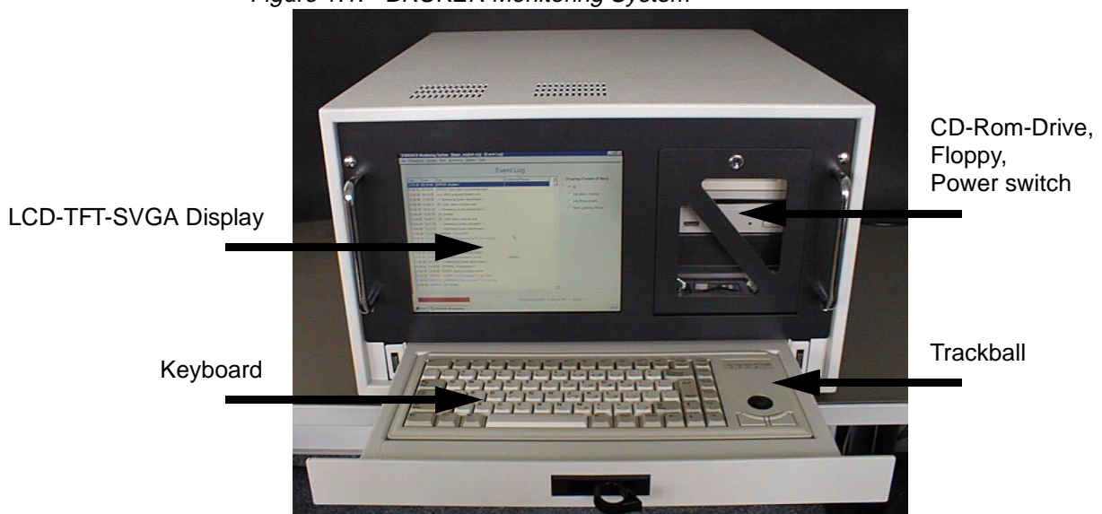
Figure 1.1. BRUKER Monitoring System
