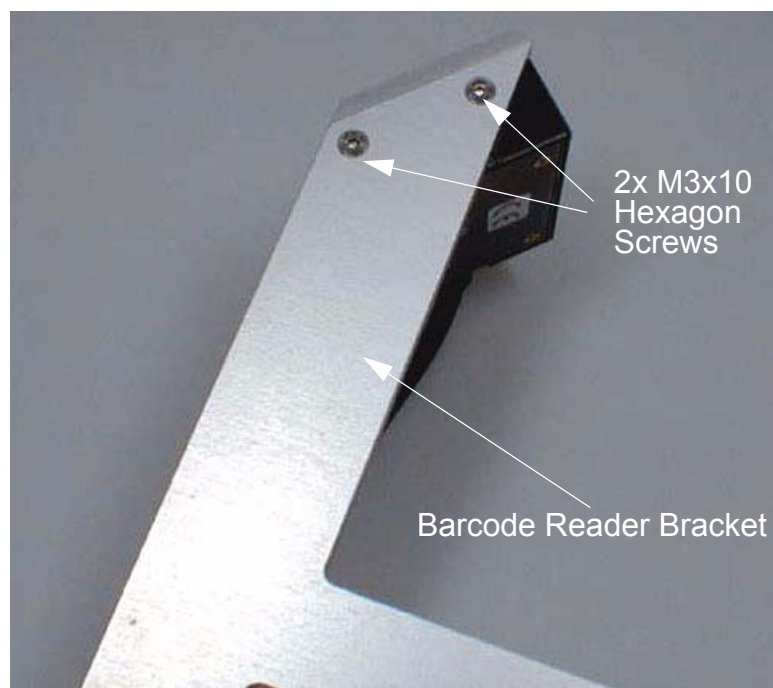
Figure 3.1. Mounting the Barcode Reader to the Bracket
