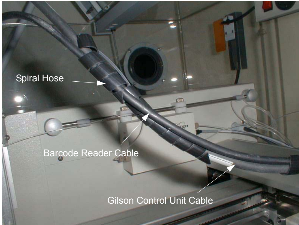
Figure 3.4. Securing the Barcode Reader Cable to the Control Unit Cable
