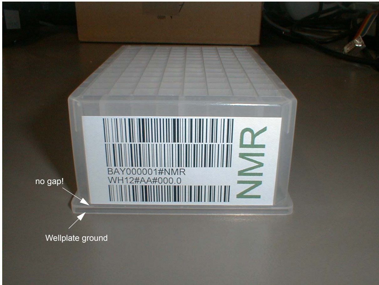
Figure 5.3. Position of a Barcode Label on a Wellplate
