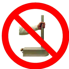
Figure 4.2. Never hold a CryoProbe at its tube!
