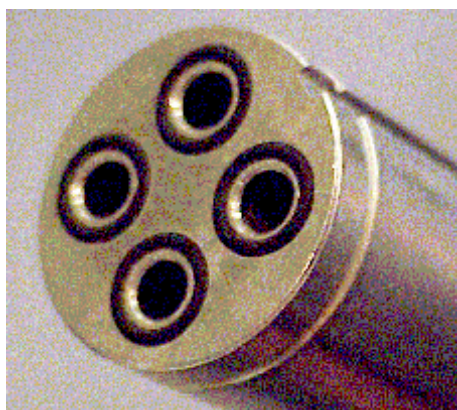
Figure 4.7. O-rings on the CryoCoupler
