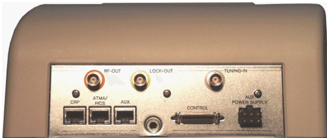
Figure 2.2. Cover Module rear view
