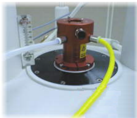
Figure 4.2. Magnet with BOSS Shim System Already Mounted
