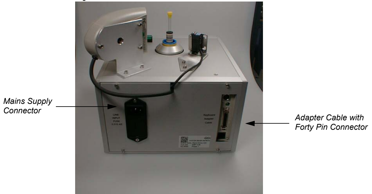
Figure 2.2. Rear Panel of the B-BCE Unit
