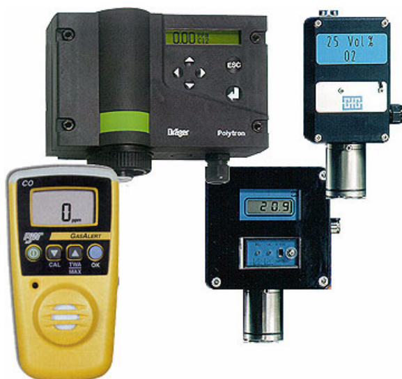
Figure 8.3. Example of some Oxygen Monitors and Level Sensors
