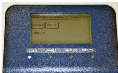
Figure 6.2: CryoCooling Unit touch screen interface and LED display
