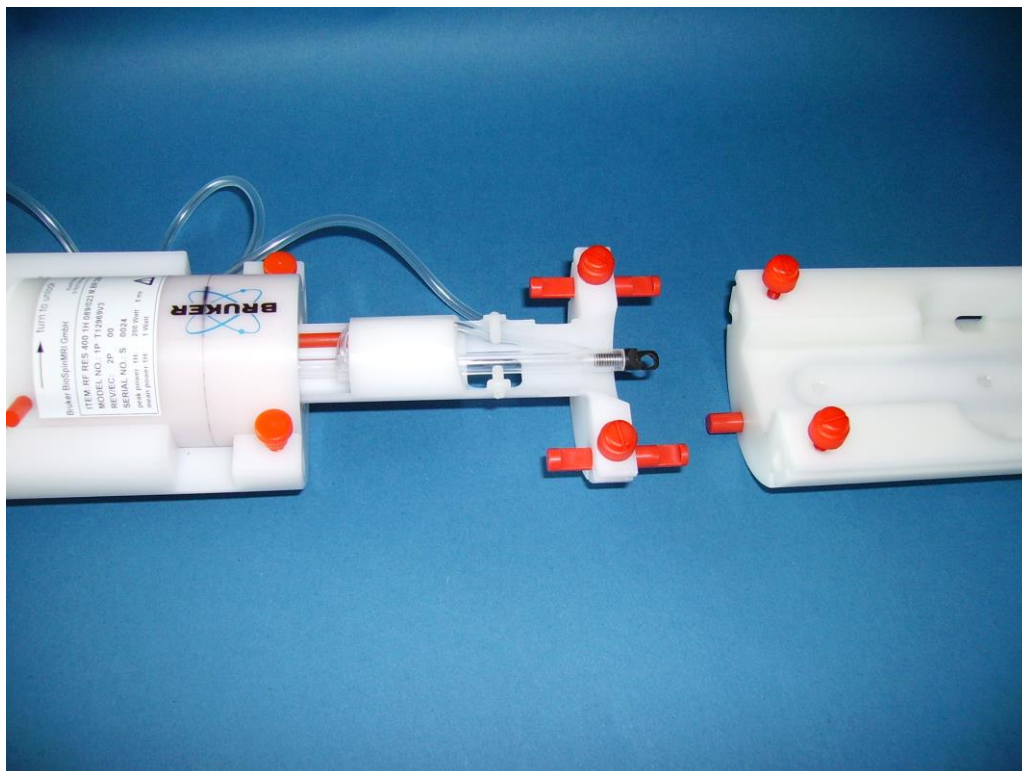
Figure 13: Mounting of the 23 mm resonator. The resonator housing has a shift mechanism to slide the resonator over the animal's head after preparation.
