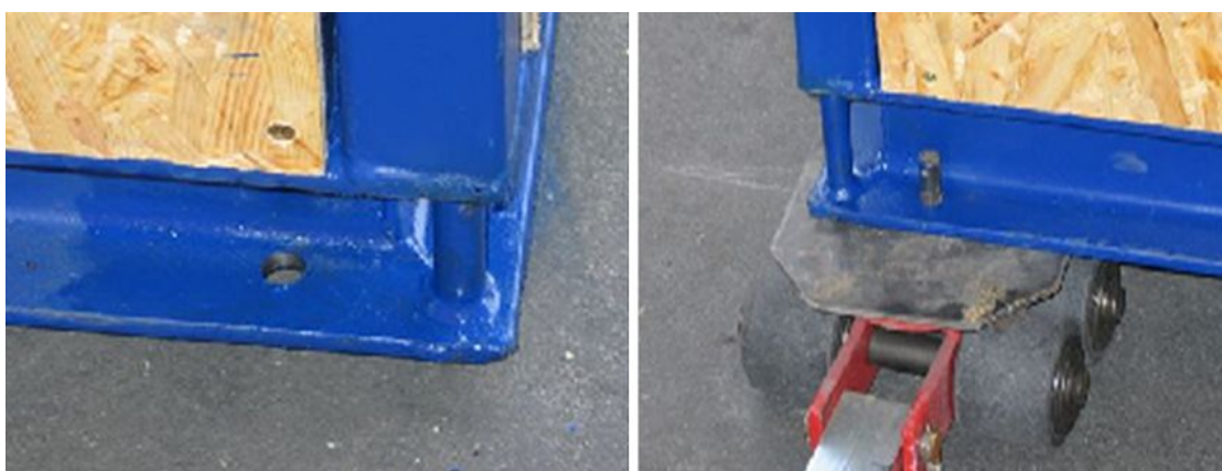
Figure 7.3: Transportation using heavy duty rollers
