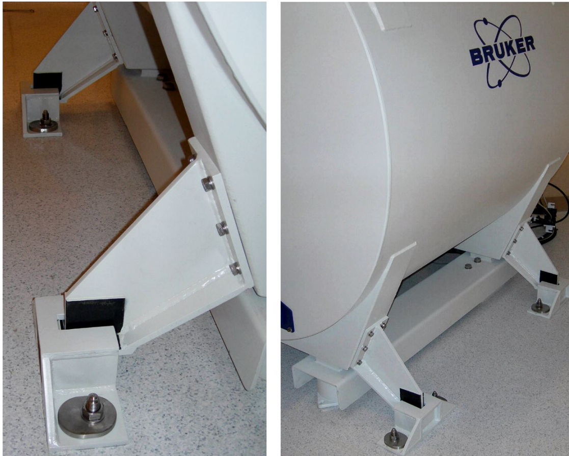
Figure 6.13: Seismic protection system at the magnet.
