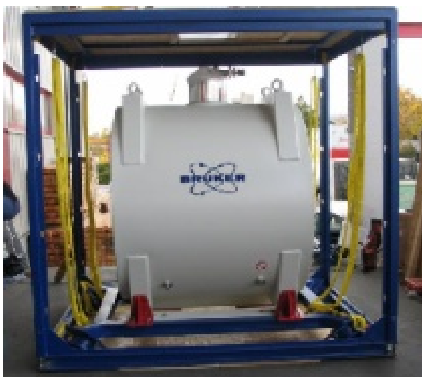
Figure 7.2: Transport pallets for air freight
