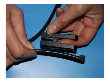
Grasp the collar with the thumb and index finger and insert the collar groves into the tracks of the clip. Use the index finger to push the collar to the end of the clip opening.
