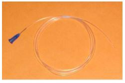
tubing. Cannulas can be constructed in a number of ways using needles, tubing and Leur connectors.
