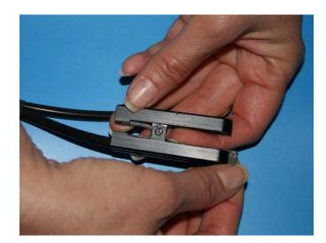
To remove the fiber, grasp the fiber with the thumb and index finger as shown. Push the fiber to move the collar away from the clip. Then grasp the collar with the thumb and index finger and remove the collar from the clip.
