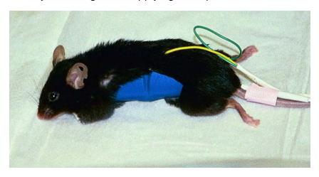
For rats, the lead does not need to extend around the entire cradle. The longer the length of wire attached to the cradle, the larger the respiration signal superimposed on the ECG waveform. At 4.7 T taping the lead on one half of the cradle gives a suitable signal. For higher field systems, less lead length coupled to the cradle maybe desirable.
