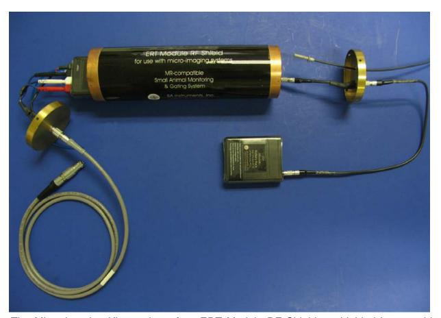
The Micro-Imaging Kit consists of an ERT Module RF Shield, a shielded Lemo cable and an assortment of in-bore sensor and sensor extension cables.
