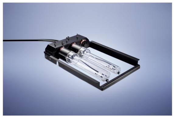
Figure 4.6: Adapter for Xtreme to support 3 Multimodal Animal Cassettes. 2 of 3 mounted.
