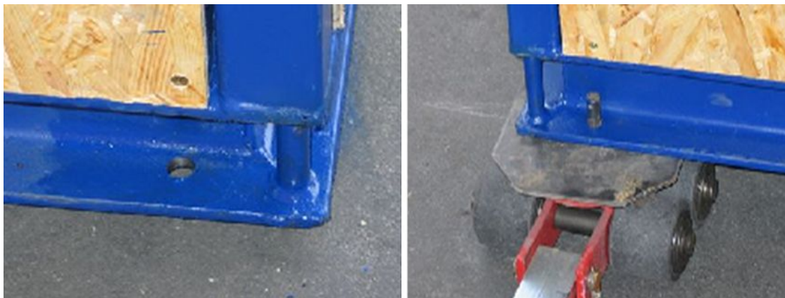
Figure 7.3: Transportation using heavy duty rollers
