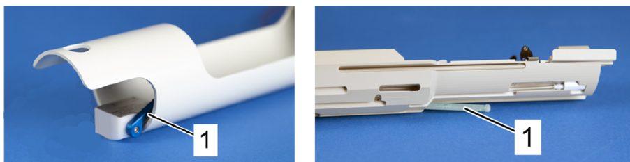
Figure 6.6: Left side: Blue lever (1) in up position. Right side: The lifting arm (1) is pushed out to lift the Animal Bed.
