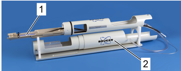
Figure 5.1: Total View of the Animal Bed and Rat Position Gauge
