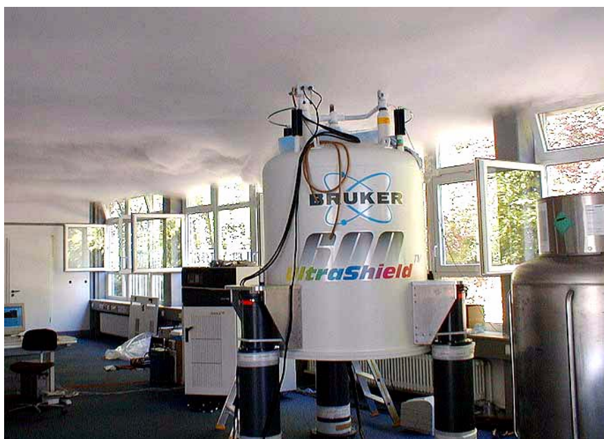
Figure 10.2. Quench at 600 MHz WB (widebore magnet)
