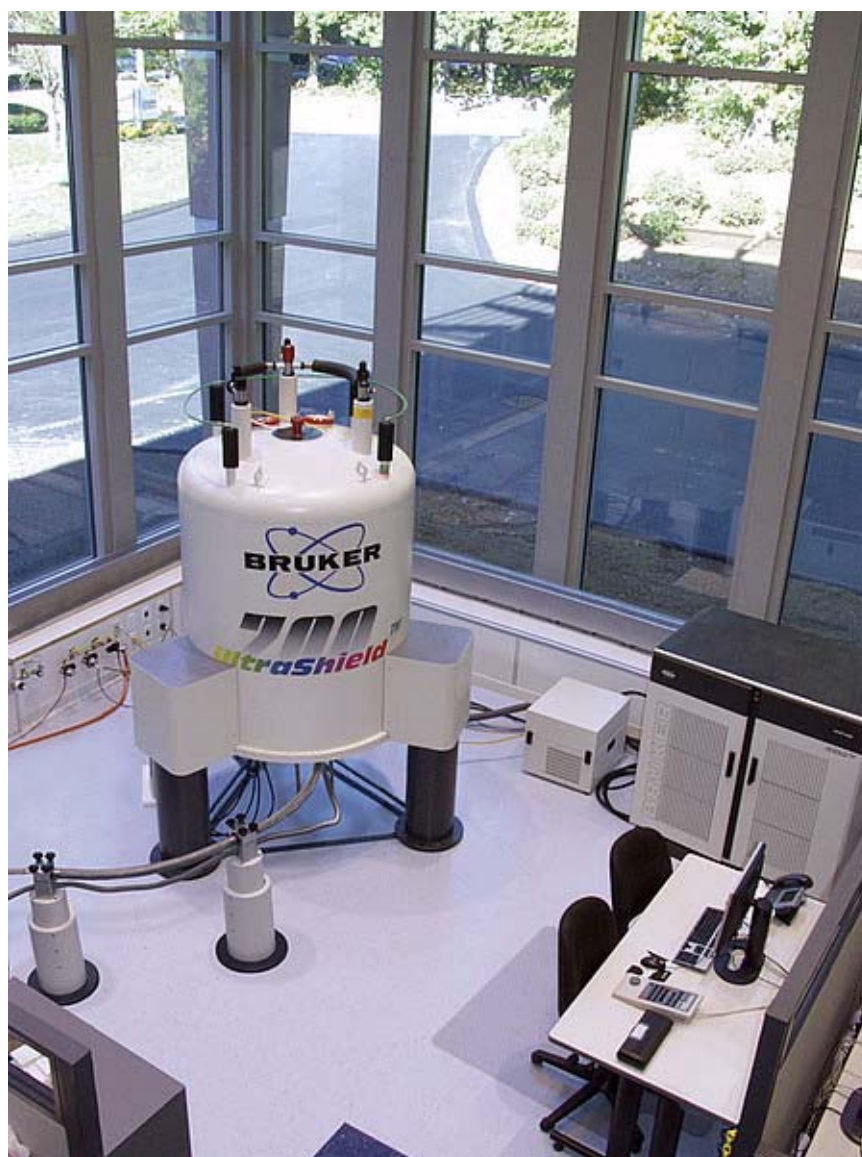
Figure 8.1. Main Units: Magnet, Cabinet, and Worktable
